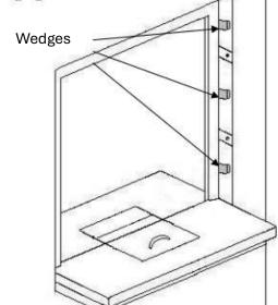
Determine the position of the transaction window with cleat.
