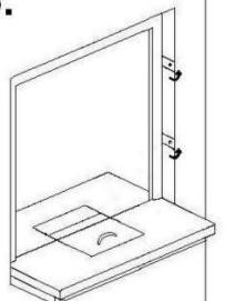
Fold back slightly assembly anchor towards the wall
